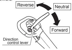
**Figure 17. Direction Control Lever**
